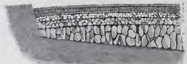
Fig. 16.—CONSTRUCTION OF ROAD IN HARTFORD CITY PARK A, Foundation; B First Layer of Broken Stones; C, Second Layer of Ditto; D, Shavings; E, Sea shore Pebbles; F, Sand
